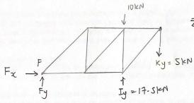
$5M_F = 0$ ,  $I_y(4) = 10(4) + 5(1)$   $I_y = 17.5 \text{ KN}$ KN
