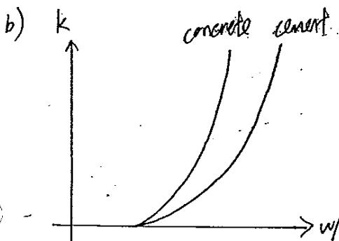
For a given w/c ratio, concrete has higher permeability coefficient.
