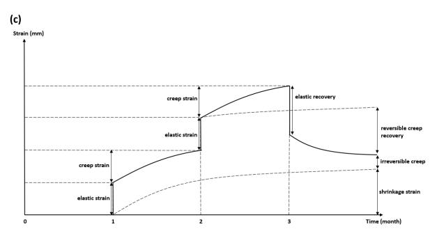
From concrete cylinder casting to one month,
