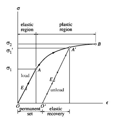
As seen in the diagram, the increase in yield point is due to grain distortion from cold work or strain hardening. The new O' falls towards the right of O, which shows that ductility is lost as permanent deformation has occurred.
