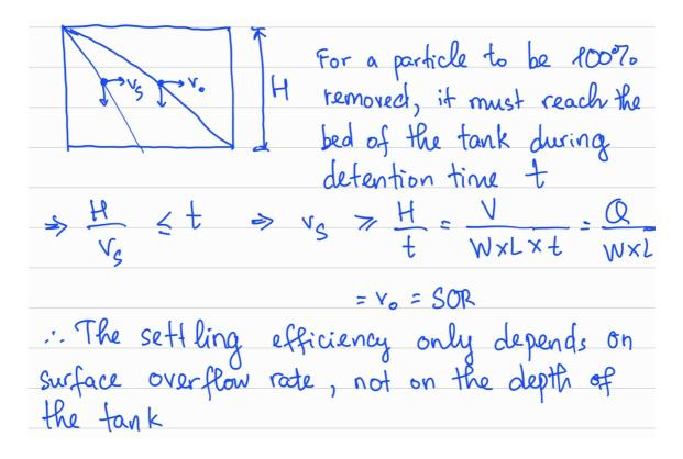
(iii) If the depth of the tank is too shallow, particles can be resuspended due to high horizontal velocity
