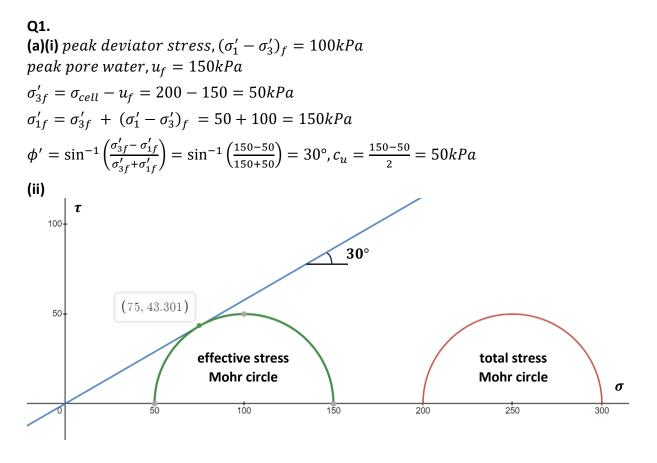
(iii) From the graph, shear stress is 43.3kPa and effective normal stress is 75kPa.
